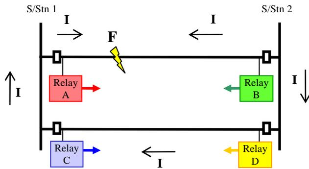
Point F is within the Zone 2 forward reach of relay D, so relay D will send a permissive signal to the remote end, relay C. Relay A will detect the fault in Zone 1, and trip instantaneously.
